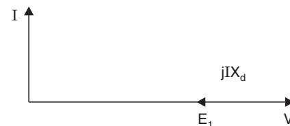
Fig. 17.23 Phasor diagram for under-excited case and P = 0 .
