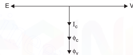
Fig. 14.56 Phasor diagram for through fault.
