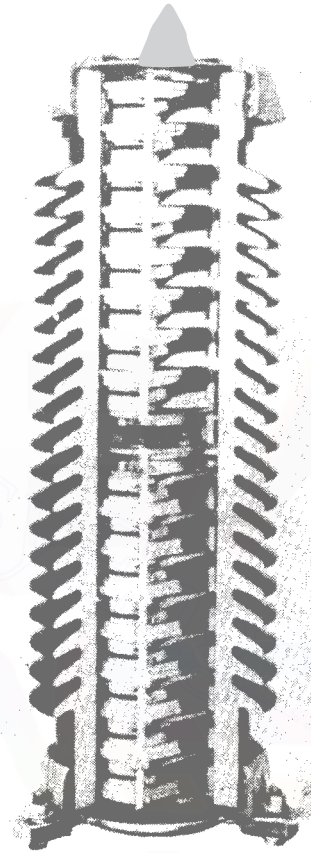
Fig. 16.11 Valve-type lightning arrester.
